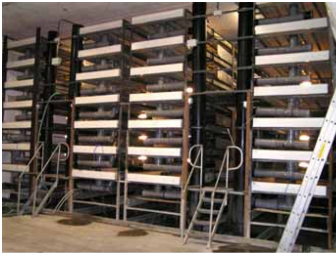
Shallow raceways being used to grow Solea solea in a recirculation on-growing system in Holland (from Andries Kamstra).
